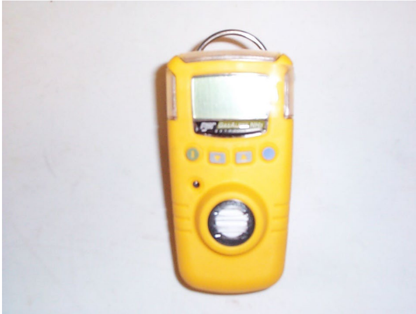
An ammonia meter with two alarms, audible and visible, shown here
