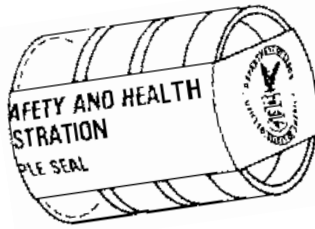
Air sampling cassette for particles ready for shipment
