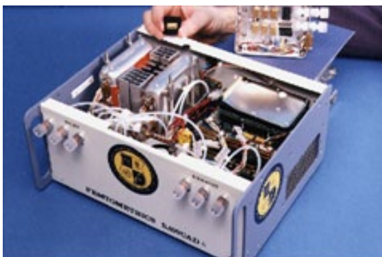
The NRL SAW sensor.
