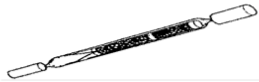
Solid sorbent tube, personal pump, lab analysis (MEASURE concentration)
