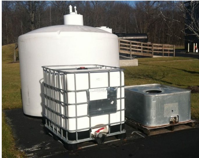
Two examples of Intermediate Bulk Storage containers in front of a bulk storage container
