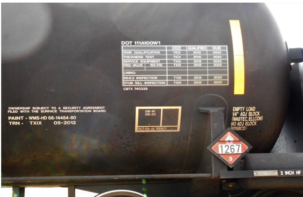
Close up of rail car placard. Use DOT ERG to identify contents. Midwest Consortium photo, courtesy of BioUrja, New Town, ND. March 2017.
