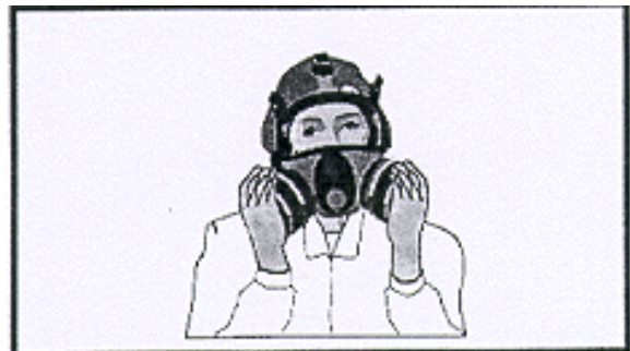
Figure: User Seal Check: worker covering inlets and inhaling (negative pressure check) from OSHA.gov
