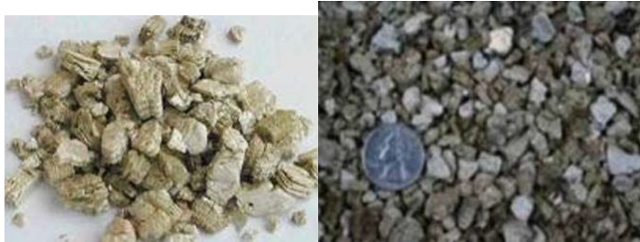
Typical Vermiculite Insulation
