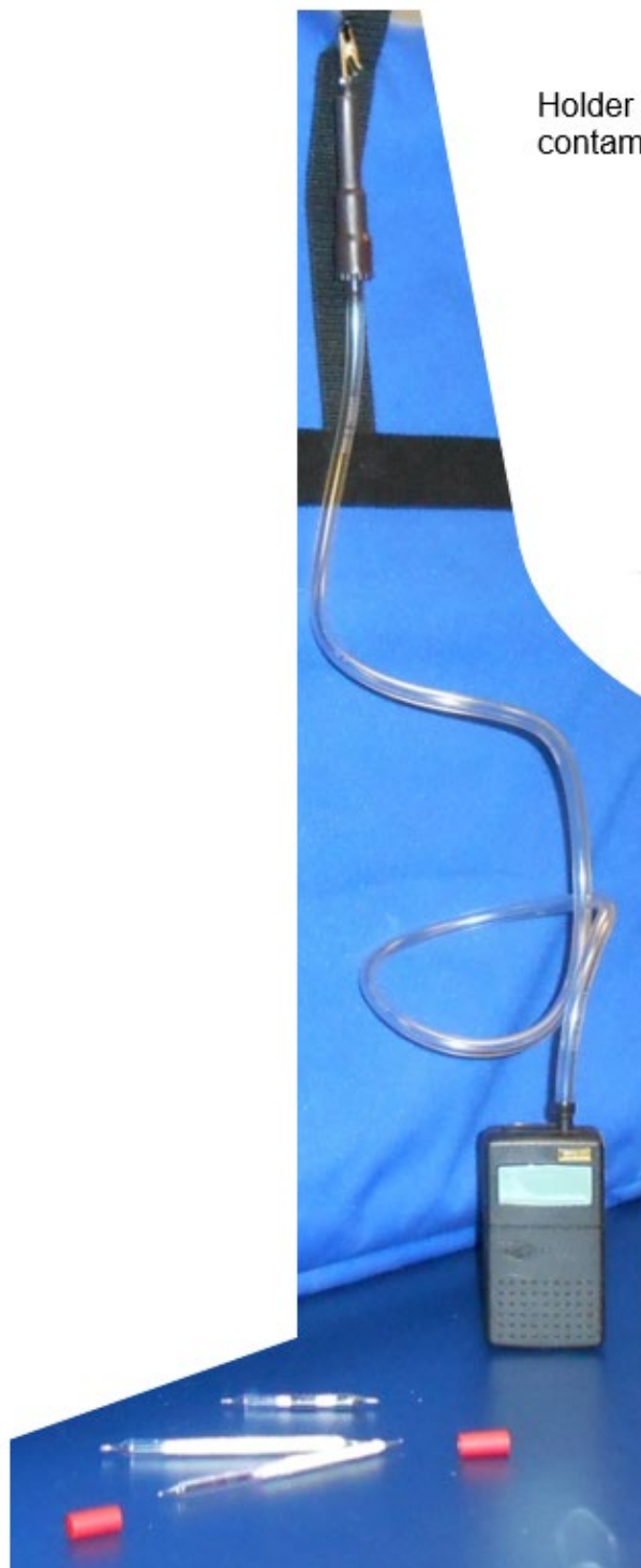
Personal monitoring sampling train for gas or vapor
