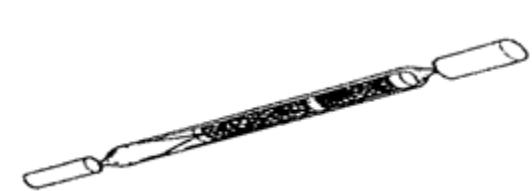
Solid sorbent tube, personal pump, lab analysis (MEASURE concentration)
