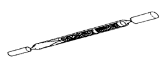
Solid sorbent tube, personal pump, lab analysis (MEASURE concentration)
