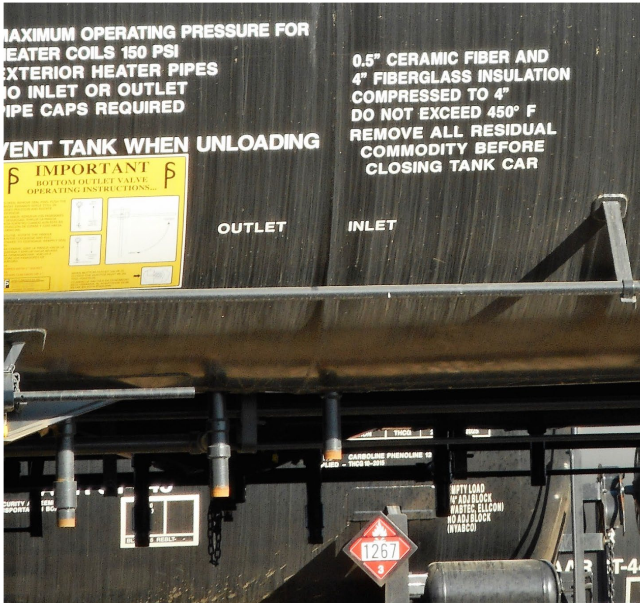
Close up of rail car placard. Use DOT ERG to identify contents. Midwest Consortium photo taken from public road in New Town, ND. November 2016.
