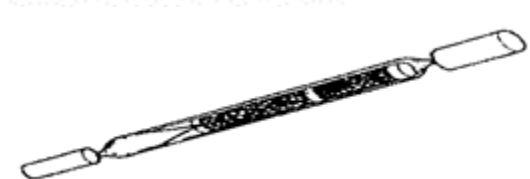
Solid sorbent tube, personal pump, lab analysis (MEASURE concentration)
